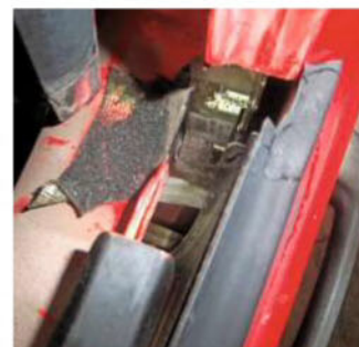
With the top weather strip removed, enough access could be gained to reach the door lock.
