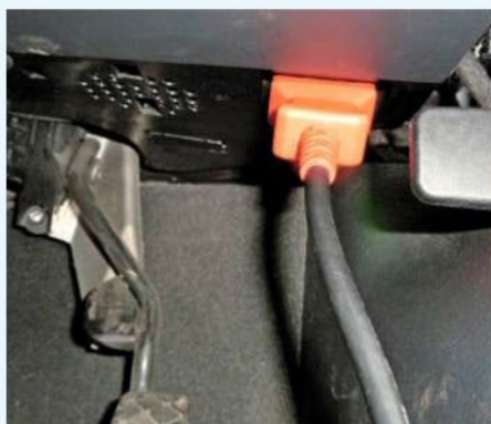
15 This Audi's diagnostic socket is located at the base of the fascia knee roll on the right-hand side of the vehicle, just above the control pedals. It is shown here with the Snap-on Verus Pro diagnostic tool connected for interrogation of the vehicle's systems.
