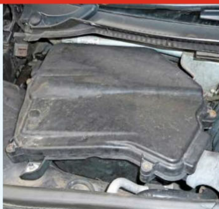
12 Beneath this plastic cover panel is the underbonnet fusebox assembly, which is best not disturbed unless absolutely necessary. Note that ingress of rainwater is likely if the cover is missing or incorrectly refitted; always check for snug fitting.
