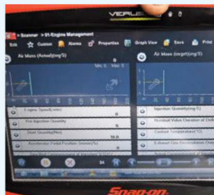
17 Live data collected by the Verus Pro tool can be invaluable when tracking down faults in the car's systems. Live data can also be very useful, and readings for mass air flow and boost pressure can quickly highlight faults.
