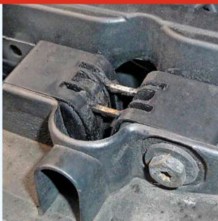
13 The bonnet switch assembly/sensor assesses whether the bonnet is fully closed. If it decides that the bonnet is still open, it will signal the ECU, in turn resulting in non-operation of the vehicle.
